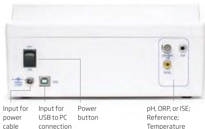
Input for power cable Input for USB to PC connection Power button Channel 2: ISE or ORP; Reference; Temperature Channel 1: pH or ORP; Reference; Temperature
