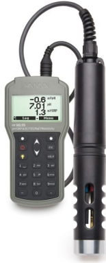
Multiparameter pH/ORP/EC/Pressure/Temperature Waterproof Meter – HI98195-20m (65.6?)
