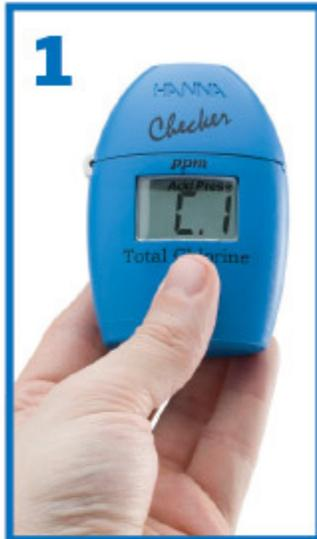
**1** "Zero" the Checker® HC as required in specific procedure
